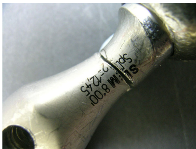
Figure 4 The fractured neck of the femoral implant.
