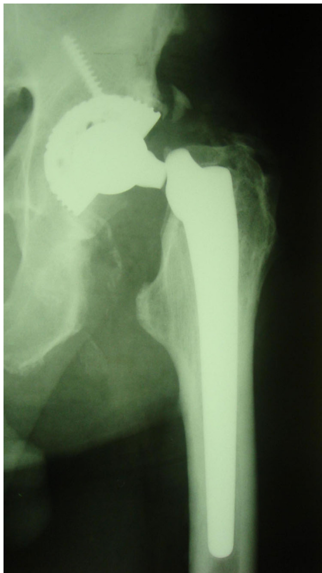
Figure 2 Fractured neck of the femoral implant prior to retrieval.
